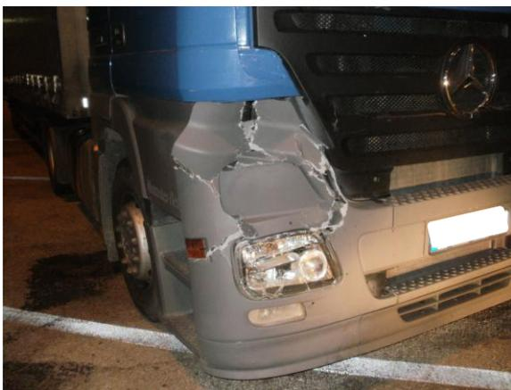
Figure 16. The damaged front right side of the tractor (P).
