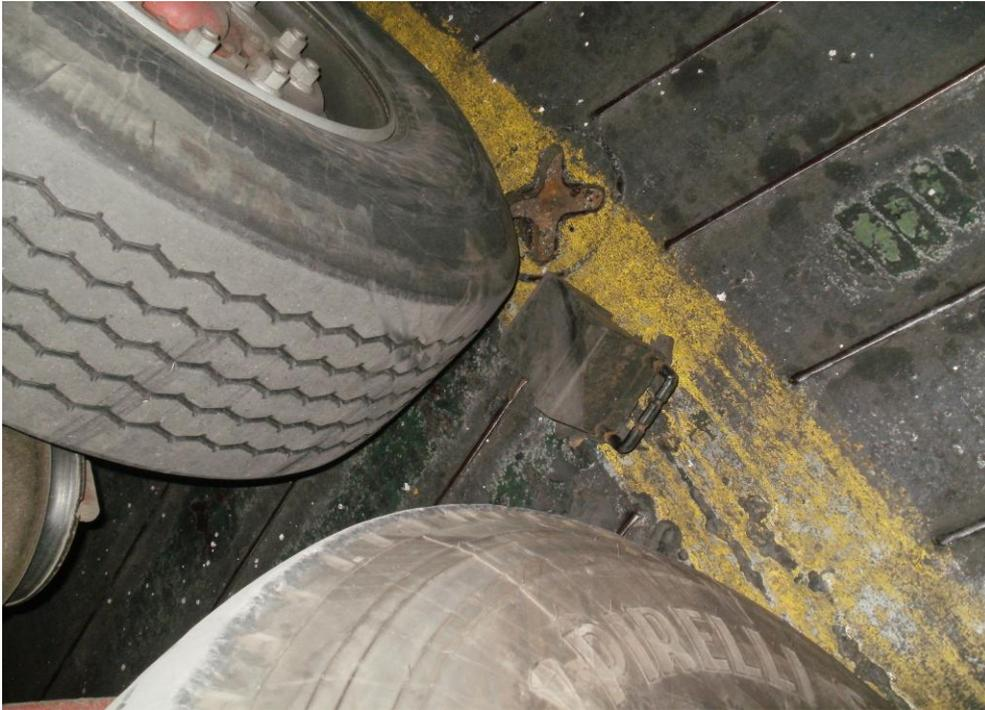
Figure 12. One of the chocks that were placed to secure the truck (S).
