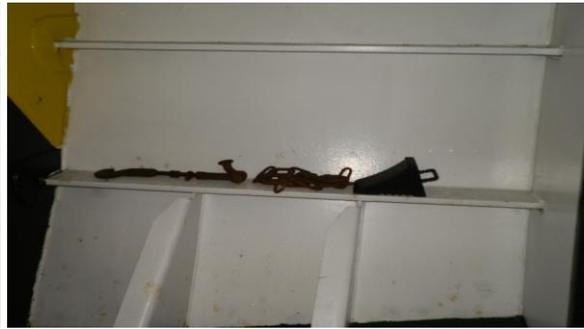
Figure 18. Securing points fitted on permanent ramp. Figure 19. The Chain lashing and rubber chocks placed at the permanent ramp.
